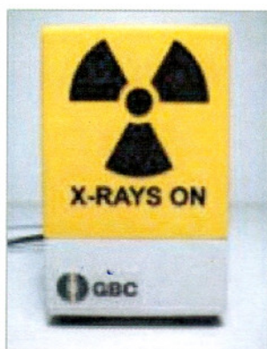
Fail-Safe X-rays ON warning Lamp.
