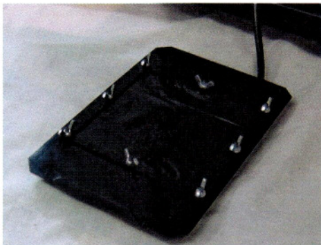
The Vacuum sample stage for contact microradiography.
